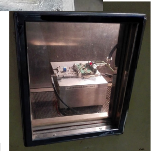
RF pallet during tests: RF and thermal measurements
