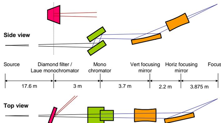
**FIGURE 1.** XALOC layout (vacuum window not shown). Diamond filter could be used as Laue mono for an ancillary branch.
