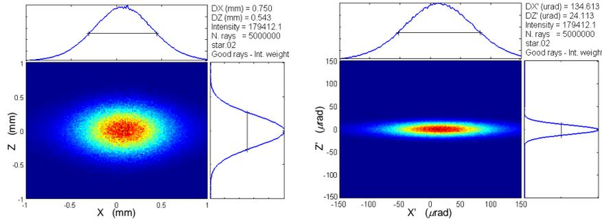
**FIGURE 4.** Raytracing simulation of the Laue diffracted beam size (*left*) and divergence (*right*) at focal point.
