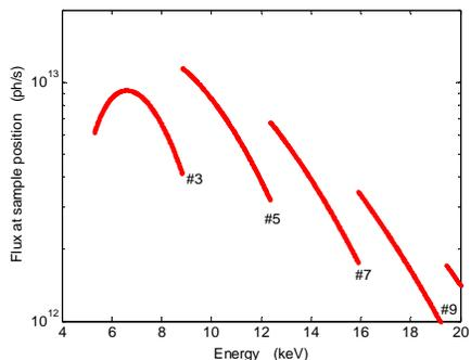
**FIGURE 3.** Calculated flux at sample position assuming a current of 250 mA in the storage ring. Calculation takes into account filter transmission (300  $\mu\text{m}$  thick, diamond), monochromator bandpass, and reflectivity and acceptance of the mirrors.
