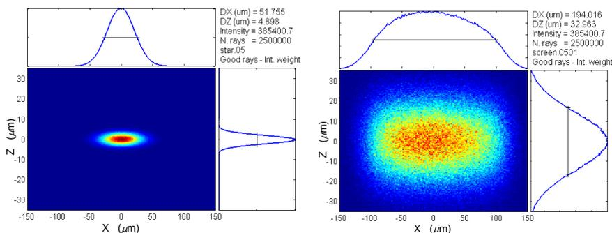
**FIGURE 2.** Simulated beam spots at focus (left), and 379 mm before (right). Photon energy is 12.658 keV.
