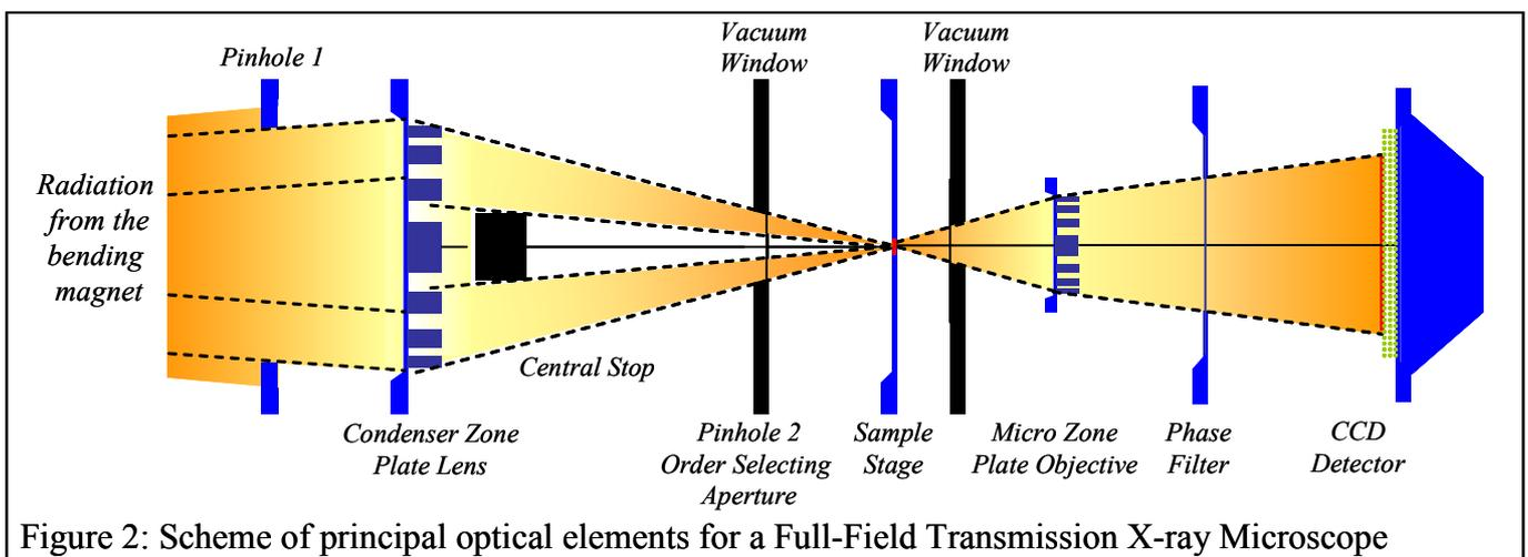
Figure 2: Scheme of principal optical elements for a Full-Field Transmission X-ray Microscope
