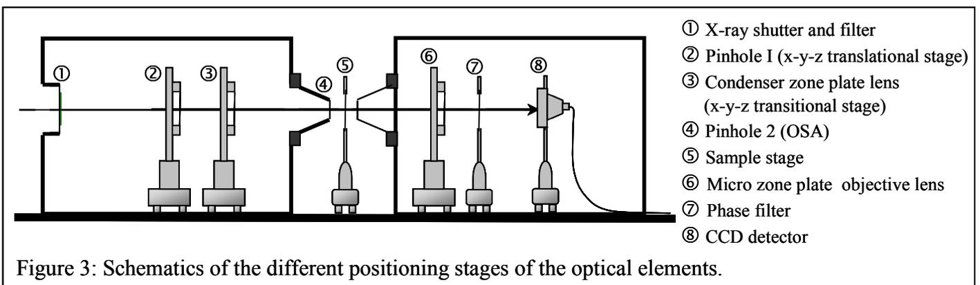
Figure 3: Schematics of the different positioning stages of the optical elements.
