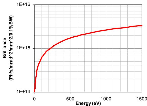
Spectral brilliance of a bending magnet source evaluated for a current of 250 mA in the ring.
